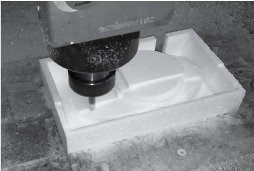
Using CNC input, the ShopBot can carve complex curves and surfaces such as an aerodynamic model helicopter fuselage. The Styrofoam for the oval fuselage was first rough-cut, then finely smoothed (here). The box surrounding the piece will be cut away. Photo by David Long.
